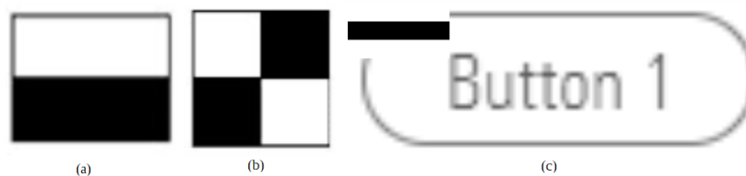
Figure 2.5. Haar-like features (a), (b) and applying one of them to the button (c).
